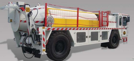
The world's most compact, low-profile mobile concrete mixer, specifically engineered for underground mining conditions.
